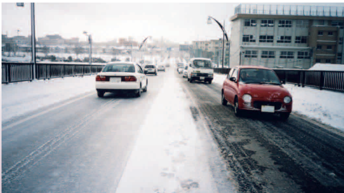
Left lane : conventional mixture. Right lane : RUBBER ROLLED ASPHALT mixture
