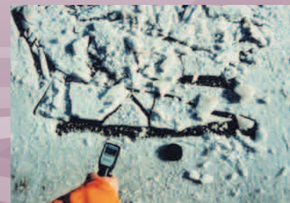
"RUBBER ROLLED ASPHALT" will allow easy removal of snow and ice.
